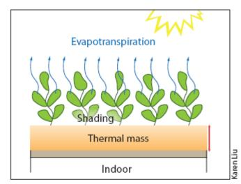
Plant shade reduces the sunlight that reaches the roof. Evapotranspiration further cools a green roof by using heat to evaporate water from the growing medium and plant surfaces
